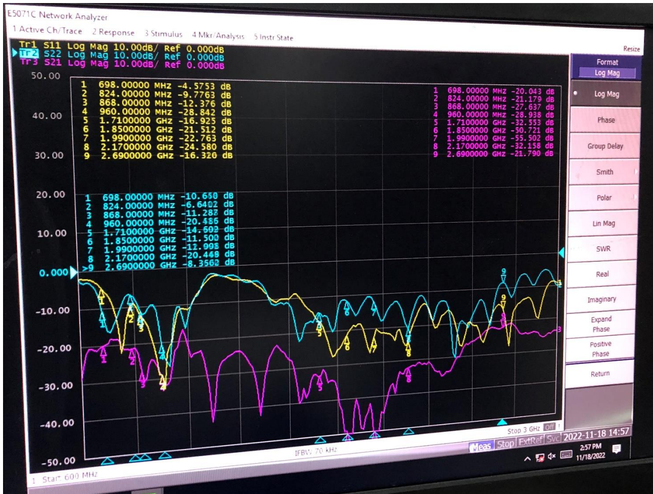
Measured S11, S22 and Isolation S21
